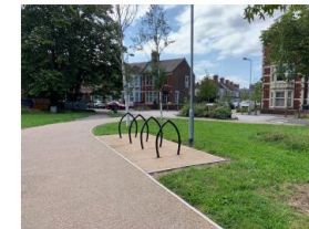
Placing cycle stands away from walls and fences ensures bikes can be correctly locked to the stand. Bespoke cycle stands can add interest to routes. Designs should consider different styles of cycle.
